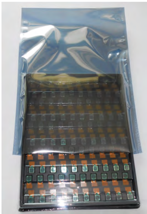
Put Tray into Anti-Static Bag
